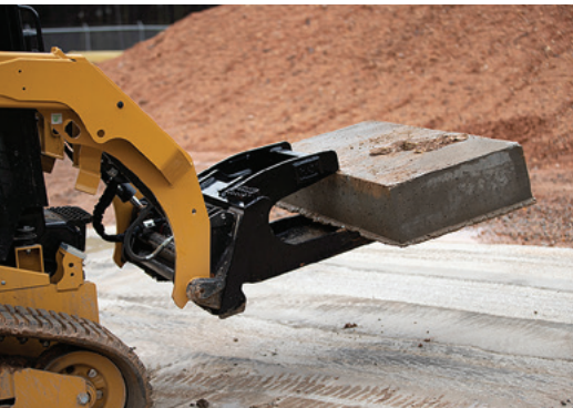
Concrete Slab Bucket
